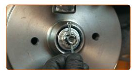
Install the cap of the hub nut. Use a hammer.
