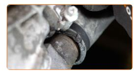
Drain the coolant from the engine.
