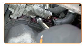
Remove the thermostat housing.
