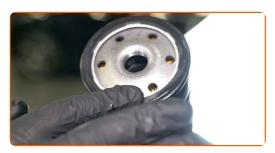
Screw the new filter into its place. Use the 74-15F socket. Use a torque wrench. Tighten it to 25 Nm torque.
