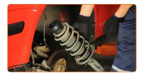
Screw the top fastening of the shock strut mount. Use a drive socket #21. Do not tighten it.
