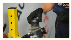
Tighten the shock strut piston rod nut. Use a drive socket #20. Use a torque wrench. Tighten it to 60 Nm torque.
