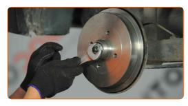
10 Remove the brake drum.
