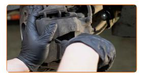
10 Remove the brake caliper.
