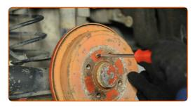
Remove the brake drum.
