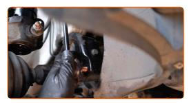
Tighten the fastener connecting the stabilizer link to the shock strut. Use a drive socket #17. Use a torque wrench. Tighten it to 40 Nm torque.
