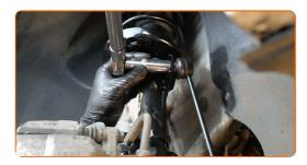
Tighten the fastener connecting the stabilizer link to the stabilizer bar. Use a drive socket #17. Use a torque wrench. Tighten it to 40 Nm torque.
