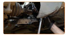
Treat all joints of the stabiliser link. Use copper grease.
