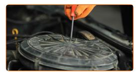
Release the air filter cover clips.
