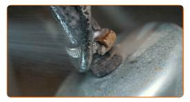
Loosen the fastening clamps of the fuel filter pipes. Use a flat screwdriver.
