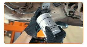
13 Install the fuel filter bracket.
