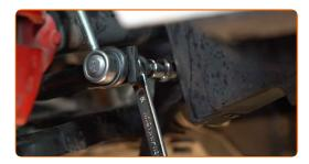
Tighten the fastener connecting the stabilizer link to the shock strut. Use a combination spanner #18. Use XZN #6. Use a torque wrench. Tighten it to 65 nm torque.
