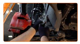
Tighten the fastener connecting the stabilizer link to the stabilizer bar. Use a combination spanner #18. Use XZN #6. Use a torque wrench. Tighten it to 65 nm torque.
