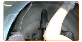
Screw in the locker fasteners. Use Torx T25. Use a ratchet wrench.
