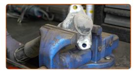
Remove the shock absorber mount cap. Use a crowbar.
