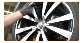
Clean the lower shock absorber fastener. Use a wire brush. Use WD-40 spray.
