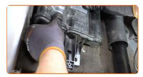
Tighten the charcoal canister fastener. Use a drive socket #13. Use a torque wrench. Tighten it to 12 Nm torque.
