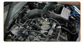
9 Unscrew the spark plugs. Use the spark plug socket #16. Use a ratchet wrench.
