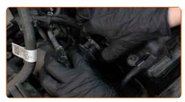
Disconnect the vacuum hose from the air filter housing.
