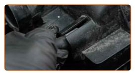
Connect the crankcase breather hose to the air filter housing.
