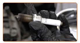
Apply a thin layer of a special high temperature anti-seize lubricant to the threads of the new spark plugs.
