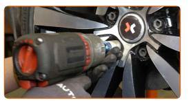
41 Lower the car and working in a cross order, tighten the wheel bolts. Use wheel impact socket #17. Use a torque wrench. Tighten it to 120 Nm torque.
