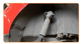
Remove the protective cap of the shock absorber mount.
