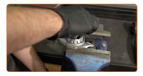
Tighten the shock absorber rod nut. Use a drive socket #16. Use a shock absorber socket DD№6. Use a torque wrench. Tighten it to 25 nm torque.
