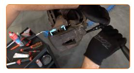
11 Remove the brake caliper.
