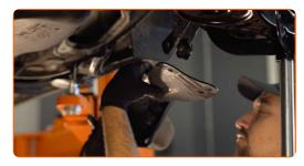
Unscrew the bracket fastening to the arm. Use a drive socket #18. Use a ratchet wrench.
