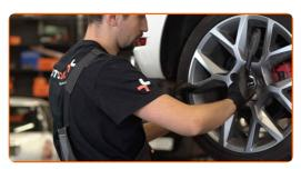
Replacement: rear suspension lower trailing arm – SEAT Leon Hatchback (1P1). AUTODOC recommends:
