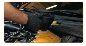
Pour coolant in the coolant reservoir.
