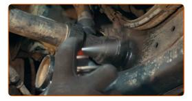
Disconnect the coolant pipe retaining clip.
