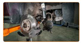
Replacement: strut mount – SEAT Leon Hatchback (1M1). Tip:
