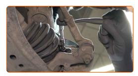
Remove the caps from the brake caliper guide pin boots. Use a crowbar.
