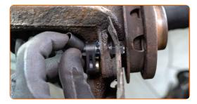
Tighten the fastener that connects the ABS sensor to the steering knuckle. Use HEX No.H5. Use a torque wrench. Tighten it to 6 Nm torque.
