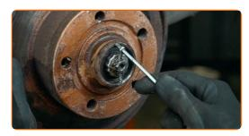
Unscrew the hub nut. Use a drive socket #24. Use a tap wrench.
