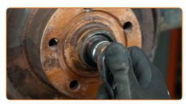
Remove the brake disc assemled with the wheel hub bearing. Use a crowbar.
