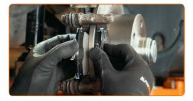
Install the brake caliper and fix it. Use a combination spanner #15. Use a drive socket #13. Use a torque wrench. Tighten it to 35 Nm torque.
