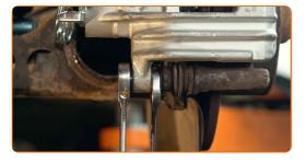
Remove the brake caliper. Use a crowbar.
