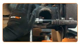
Remove the caliper bracket.
