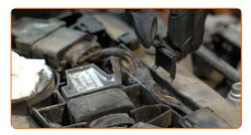
Unscrew the fastener of the chassis (ground) terminal of the ignition coils. Use a drive socket #10. Use a ratchet wrench.
