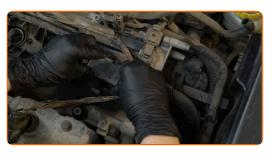
Install the ignition coils to the spark plug wells. Make sure you hear a click indicating that it is locked in place.
