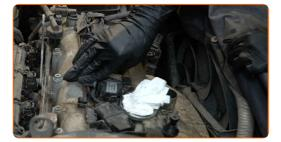
Tighten the chassis (ground) terminal of the ignition coils. Use a drive socket #10. Use a ratchet wrench.
