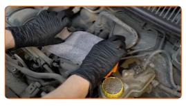
Take out the ignition coil from the spark plug well. Use a crowbar.
