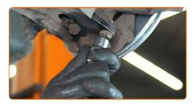
Attach the transmission sensor connector.
