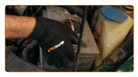
Unscrew the fasteners of the battery tray. Use a drive socket #10. Use a ratchet wrench.
