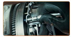
Align the clutch disc. Use a crowbar.
