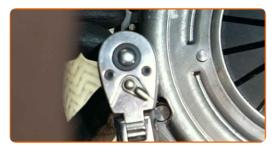
Install the engine flywheel locking tool. Use a clutch tool kit.
