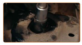
Unscrew the fastener that connects the gearbox mount to the car body. Use a drive socket #13. Use a ratchet wrench.
