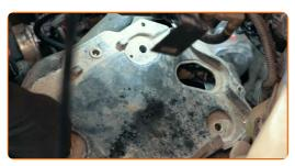
Screw in the battery tray fasteners. Use a drive socket #10. Use a ratchet wrench.
