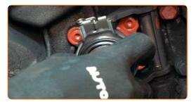
Unscrew the pressure plate fasteners. Use 12-point socket No.9. Use a ratchet wrench.
