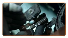
Remove the gear shift cable retaining clip. Use a flat screwdriver.
