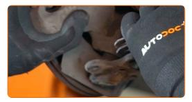
Detach the driveshaft from the steering knuckle.
