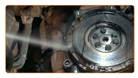
Install the new pressure plate together with the clutch disc.
