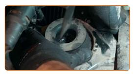
Screw in the fasteners that connect the gearbox mount to the car body. Use a drive socket #18. Use a ratchet wrench.
