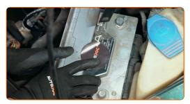
Screw in the battery fastener. Use a drive socket #13. Use a ratchet wrench.
