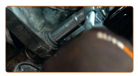
Tighten the fastener of the cable bracket. Use a drive socket #16. Use a torque wrench. Tighten it to 22 Nm torque.
