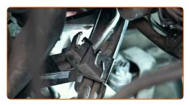
Screw on the ground wire fastener. Use a combination spanner #13.
