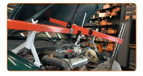
Unscrew the fastener of the cable bracket. Use a combination spanner #16.
