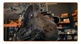
Remove the release bearing. Use a crowbar.
