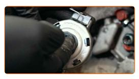
63 Install the new release bearing.
