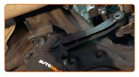
Screw in the fasteners that connect the gearbox mount to the subframe. Use a drive socket #13. Use a ratchet wrench.
