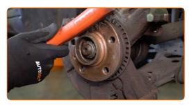
25 Install the brake disc.
