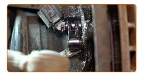
Unscrew the brake caliper fastening. Use HEX No.H7. Use a ratchet wrench. Use a tap wrench.
