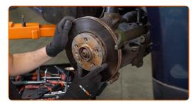
Tighten the brake disc fastening. Use Torx T30. Use a torque wrench. Tighten it to 6 Nm torque.
