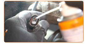
Attach the ABS sensor connector.
