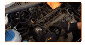
7 Unscrew the oil filler neck. Remove the oil filler neck.
