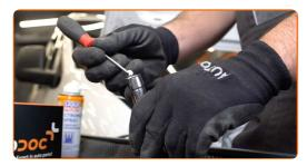
Plug in the ignition coil connector.
