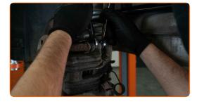
11 Remove the brake caliper.
