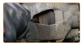
Remove the brake caliper.
