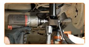
9 Remove the fastening bolt.
