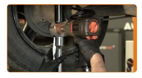
Remove the fastening bolt.
