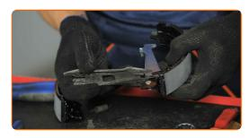
20 Install the retaining spring of the brake pads.
