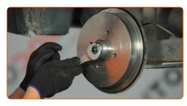
10 Remove the brake drum.
