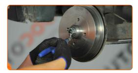
Unscrew the wheel hub axle nut. Use a combination spanner #24.
