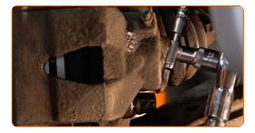
Clean the brake hose mounting seat on the brake circuit pipe. Clean the mounting seat of the brake hose on the brake caliper. Use a brake cleaner.
