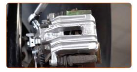
Attach the brake caliper bleed screw cap.
