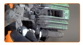
Remove the brake caliper. Use a crowbar.
