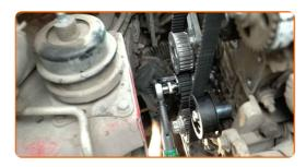
Remove the camshaft gear locking tool.
