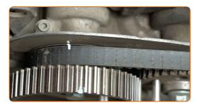
Remove the timing belt tensioner pulley. Use a drive socket #16. Use a ratchet wrench.
