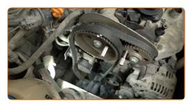
Clean the fastener of the timing belt idler pulley. Use a wire brush. Use WD-40 spray.
