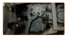
Tighten the crankshaft pulley fastener. Use 12-point socket No.21. Use a torque wrench. Tighten it to 90 Nm torque.+90°
