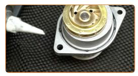
Install the water pump gasket.
