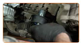
Tighten the fastener of the timing belt idler pulley. Use a drive socket #15. Use a torque wrench. Tighten it to 25 Nm torque.
