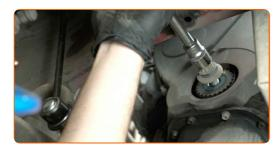
Unscrew the fasteners of the lower timing cover. Use a drive socket #10. Use a ratchet wrench.
