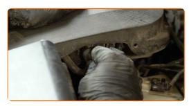
109 Remove the coolant reservoir cap.
