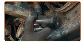
Disconnect the coolant pipe retaining clip.
