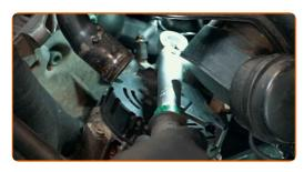
Connect the alternator connector.
