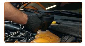
Pour coolant in the coolant reservoir.
