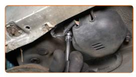
Remove the oxygen sensor housing cover.
