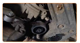
Screw in the engine mount fastener that connects it to the subframe. Use a drive socket #16.
