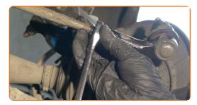
Unscrew the end fastening nut to the steering knuckle. Use a drive socket #19. Use a tap wrench.
