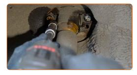
10 Remove the fastening bolt.
