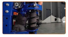
Remove the assembled shock strut.
