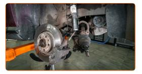
Replacement: strut mount – SEAT Ibiza IV Hatchback (6J5, 6P1). Tip:
