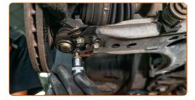
Disconnect the spherical joint from the arm.
