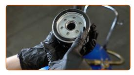
Screw the new filter into its place. Use a drive socket #30. Use a torque wrench. Tighten it to 26 Nm torque.
