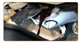
Replacement: engine oil and filter – SEAT Ibiza IV Hatchback (6J5, 6P1). Tip:
