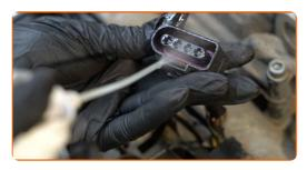
9 Plug in the connectors of the ignition coils.
