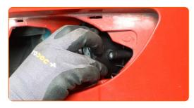
Screw in the fog light fasteners. Use Torx T20.
