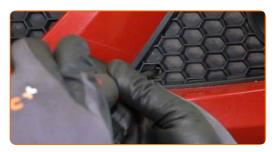
Use the masking tape to prevent plastic and painted parts of the car from being damaged.
