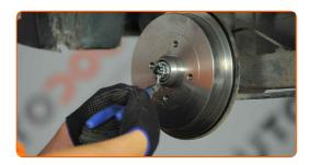
9 Unscrew the wheel hub axle nut. Use a combination spanner #24.
