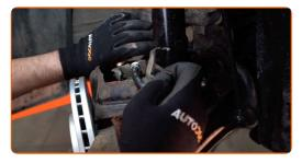
Install the brake hose retaining clip. Use a rubber mallet.
