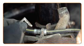
Detach the brake hose from the shock strut.
