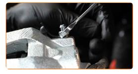
Remove the brake hose clamp.
