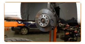
Clean the area where the brake hose is connected to the brake caliper and to the brake circuit pipe. Use a wire brush. Use a brake cleaner.
