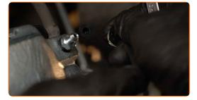
Tighten the brake caliper bleed screw. Use a drive socket #11. Use a torque wrench. Tighten it to 9 Nm torque.
