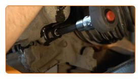
14 Remove the brake caliper.
