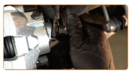
Tighten the fastener connecting the brake pipe to the brake caliper. Use a drive socket #11. Use a torque wrench. Tighten it to 35 Nm torque.
