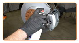
Replacement: brake caliper – SEAT Ibiza IV Hatchback (6J5, 6P1). Tip from AUTODOC experts:
