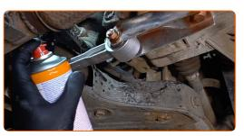
Replacement: manual gearbox oil – SEAT Ibiza III Hatchback (6L). Tip from AUTODOC:
