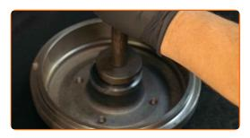
Install a new hub bearing and secure it.
