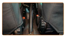
Loosen the parking brake cable. Use a combination spanner #10.
