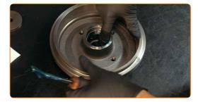
Install a new hub bearing and secure it.
