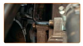
Unscrew the fastener of the viscous fan clutch. Use a combination spanner #46. Use HEX No.H8.
