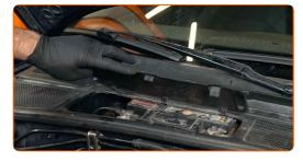
Unscrew the fasteners of the car battery terminals. Use a combination spanner #10.
