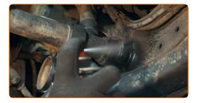
Disconnect the coolant pipe retaining clip.
